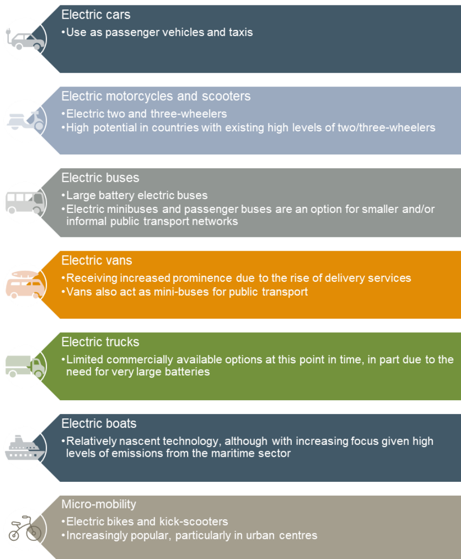
Figure 3 Overview of different types of EVs
