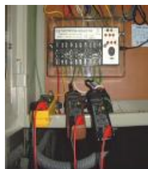
② Secondary current measurement
