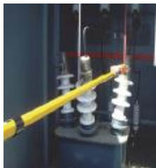
① Primary current measurement
