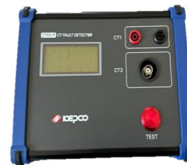
CTFD(CT Fault detector)
